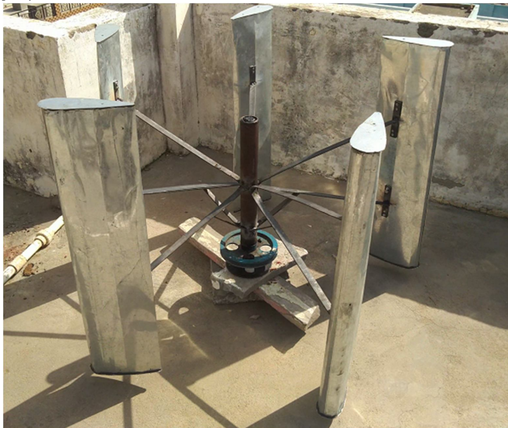
Fig:- Vertical axis wind turbine
