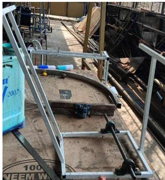
Fig 3: Initial fabrication of the mild steel chassis.
