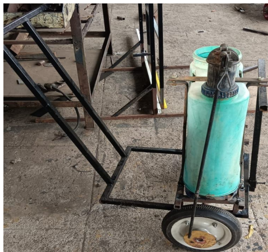
Fig 4: Integration of the 16L tank and ground-driven crank linkage.
