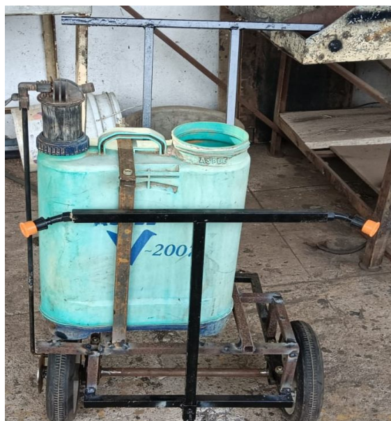
Fig 5: Final assembly showing the dual-nozzle boom.
