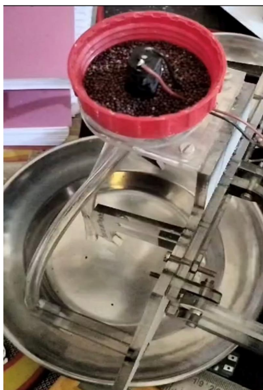
Figure 4. Actual seed sowing mechanism.
