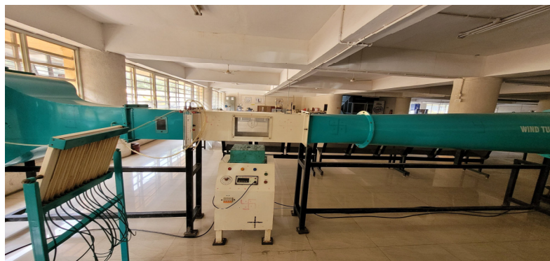
Fig. 5 Wind tunnel set-up (Test Section)
