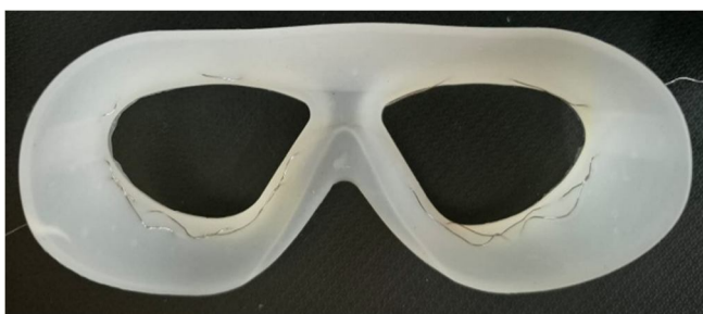
Fig. 3. Eye Mould With Integrated Heating Wire And Sensor System.
