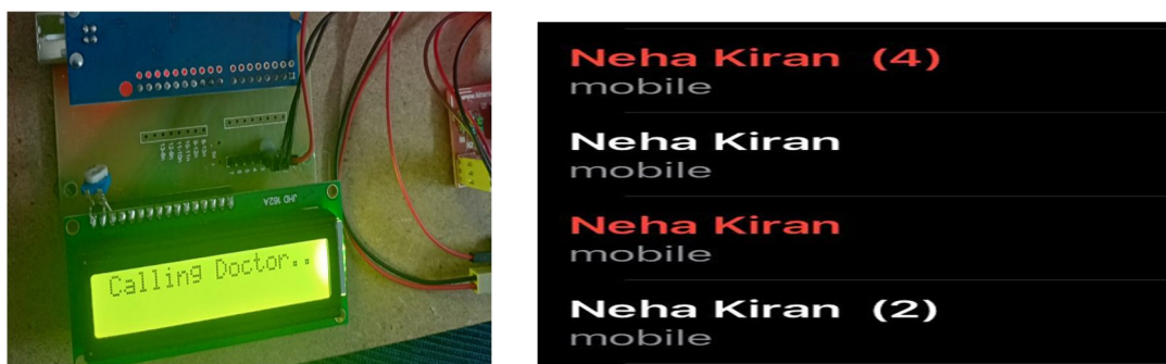
Fig 5.8 Calling the doctor if the defined thresholds reached and doctor(Neha Kiran ) received calls from the patient
