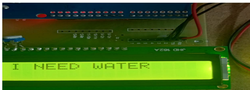
Fig 5.5 :When the flex sensor is bent ,the necessity of the patient is displayed on the LCD
