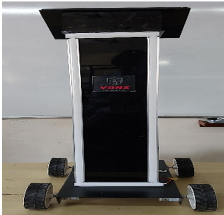
Figure 1: Line following Tour Guide AGV
