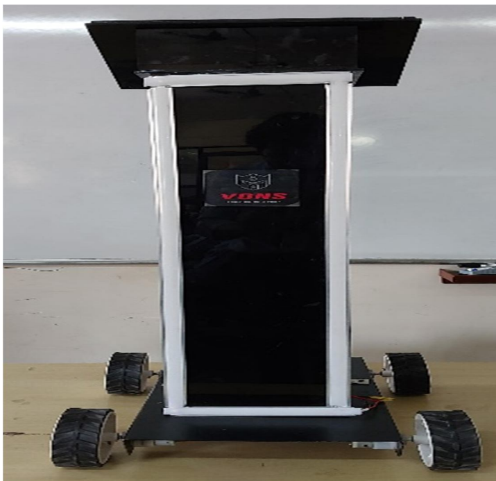
Figure 1: Line following Tour Guide AGV
