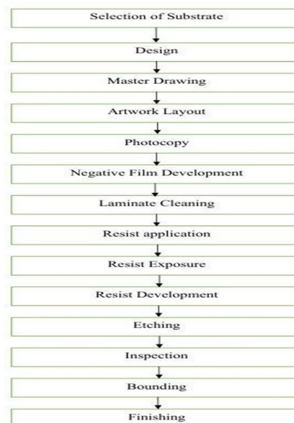
Figure 21 Flow chart of Fabrication process
