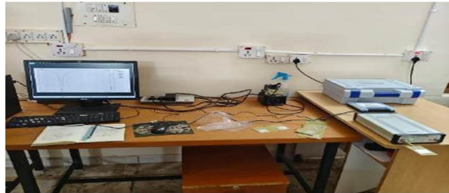
Figure 19 Taking readings of Antenna with help of VNA
