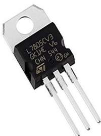
Fig.4: Voltage Regulator (LM 7805)
