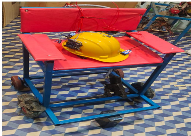
Fig. 9 Fabrication of head tilt controlled wheelchair
