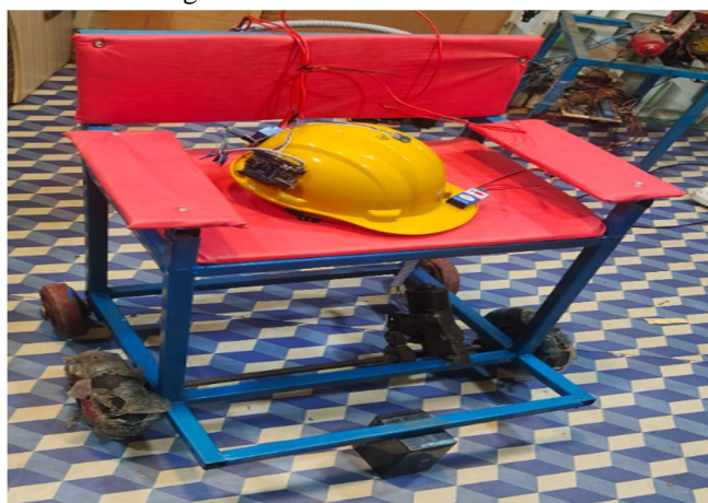
Fig. 9 Fabrication of head tilt controlled wheelchair
