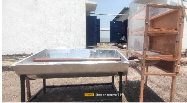
Fig 11: Fabricated PTC Solar Dryer
