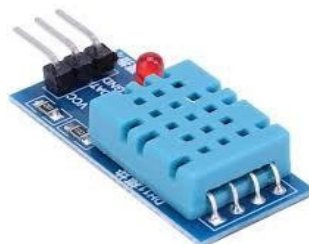
Fig 8: Temperature and Humidity sensor
