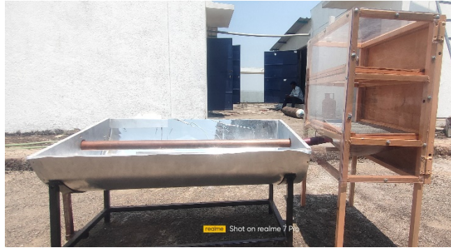
Fig 11: Fabricated PTC Solar Dryer
