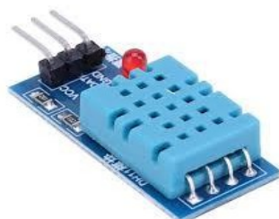
Fig 8: Temperature and Humidity sensor
