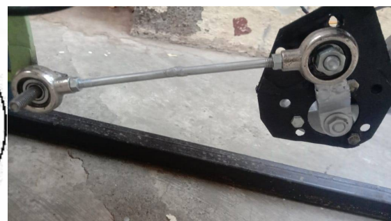
Fig: Single slider crank mechanism
