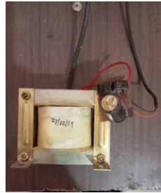
Fig : Step down transformer
