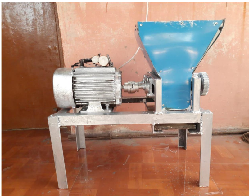
Fig 8.1 Actual Model Of Plastic Shredding Machine
