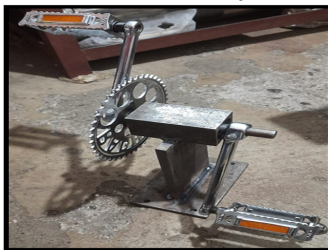
Fig 1 Lower housing with shaft and bigger sprocket
