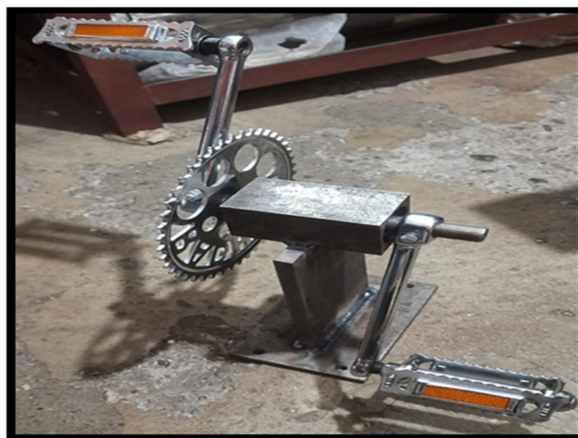
Fig 1 Lower housing with shaft and bigger sprocket
