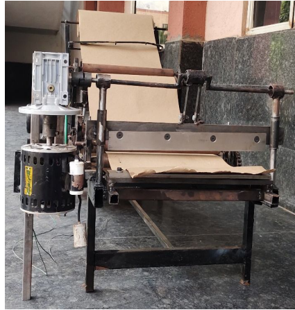
Fig.3.1 Front cutting assembly
