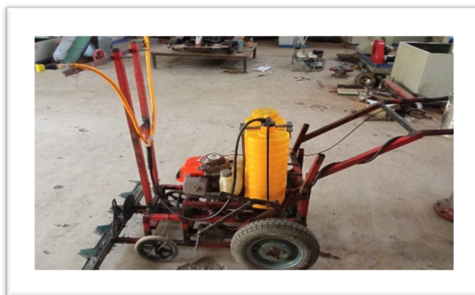
Figure 1: Multi nozzle spray machine
