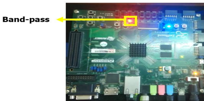
Figure 12. Band-pass filter Mode LED representation on board
