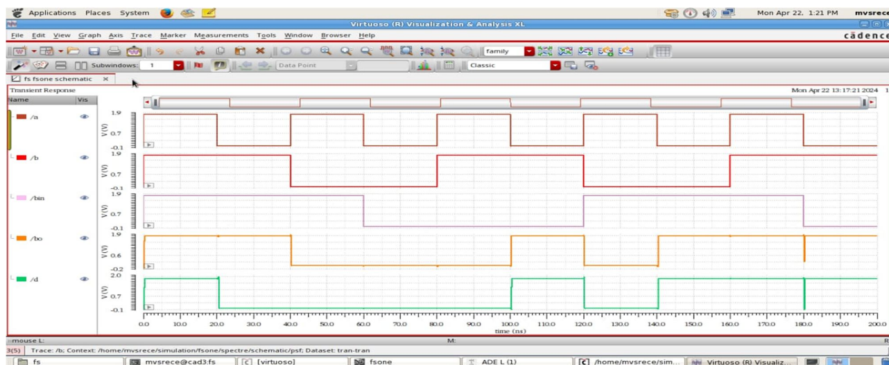
Fig.8 Output of 20T full subtractor
