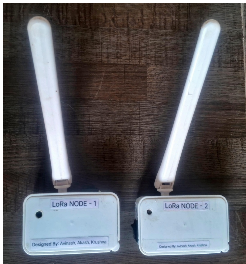
Fig. 4. Final assembled LoRa Mesh Nodes with custom weatherproof enclosure.
