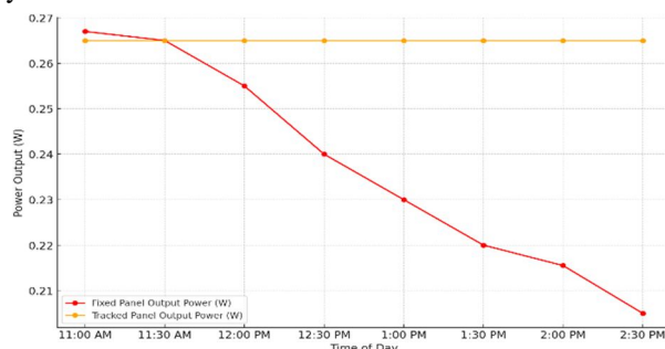
Graph 3: Power Output (W) vs Time of Day for Fixed and Tracked Solar Panels
