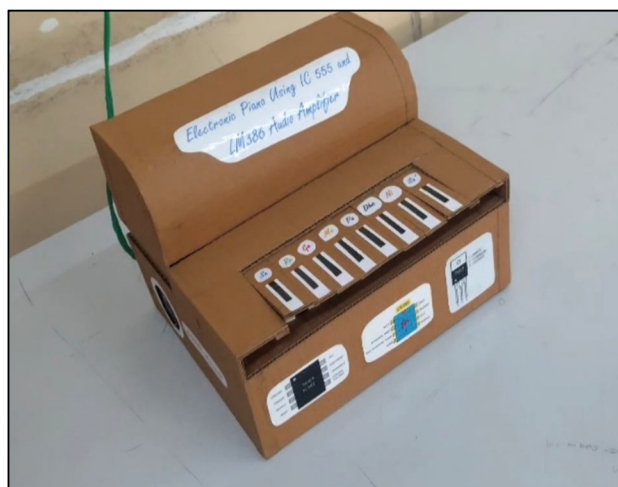
Fig. 10: Final Assembled Electronic Piano — Complete Hardware Product
