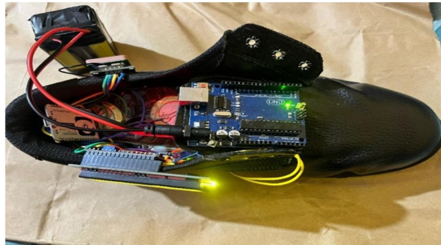
Fig:5 Circuit connected to Shoe
