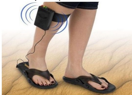
Fig:2 Signal transceiver for the metal detection sensor integrated in the footwear.
