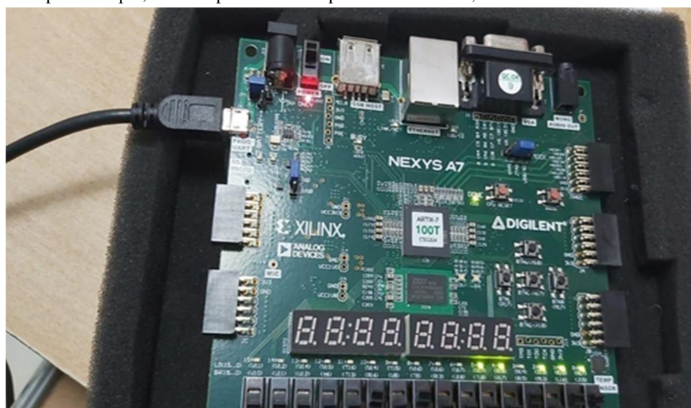
Fig. 11 Radix-8 multiplier with two positive values after FPGA implementation.
