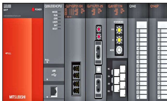
Fig. no: 2.2 Mitsubishi Q-SERIES PLC Controller.
