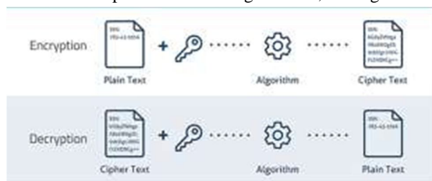
Figure – 1: Basic Block Diagram of Encryption andDecryption
