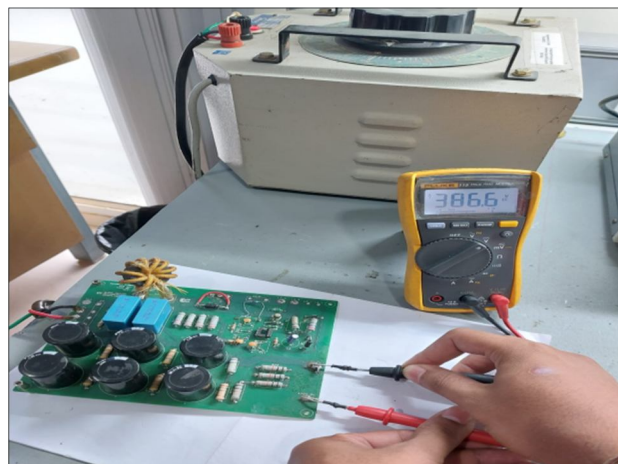
Fig. 3(a) Boost PFC Converter Board Top-View With the 230 V AC Input And Fig. 3(b) With the 386.6V DC output
