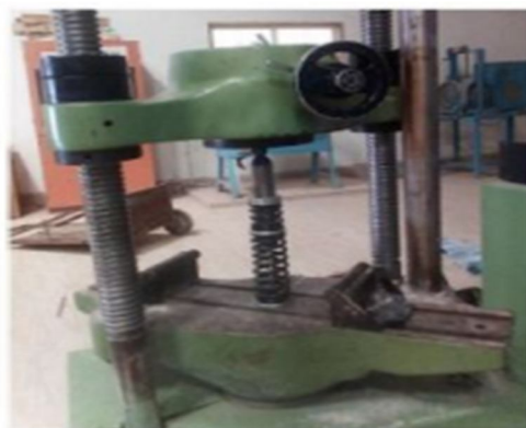
Fig 7.1: Test conducted on UTM of shock absorbers
