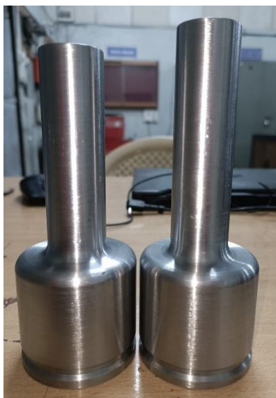
Fig. 4 Geometry after lathe machining
