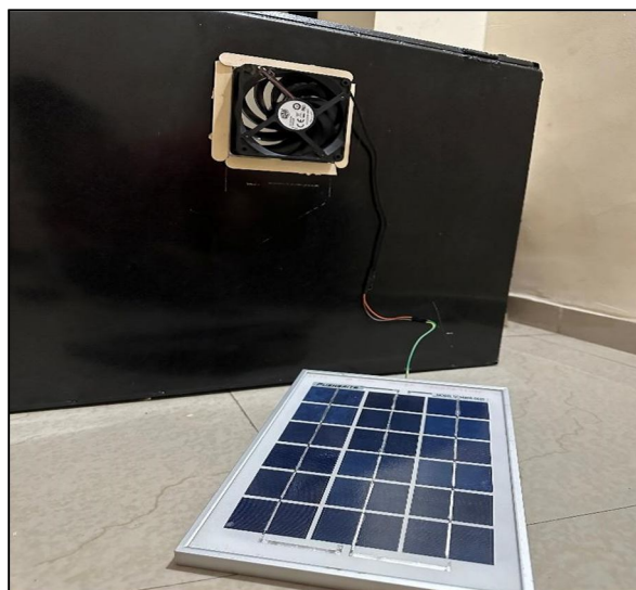
Fig. 7. Solar panel and 12V battery configuration for powering the exhaust fan and enabling autonomous operation.
