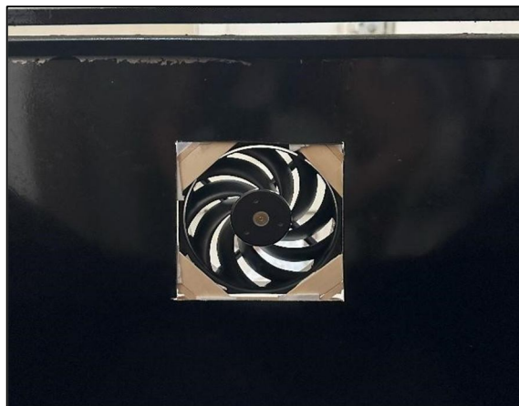
Fig. 5. Rear view of the mounted 12V exhaust fan enabling forced air convection.
