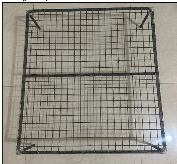
Fig. 6. Stainless steel mesh tray used for supporting fig samples during drying.
