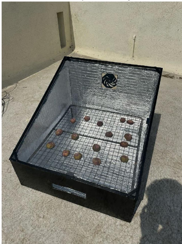
Fig. 8. Fully assembled solar dryer placed outdoors for deployment.
