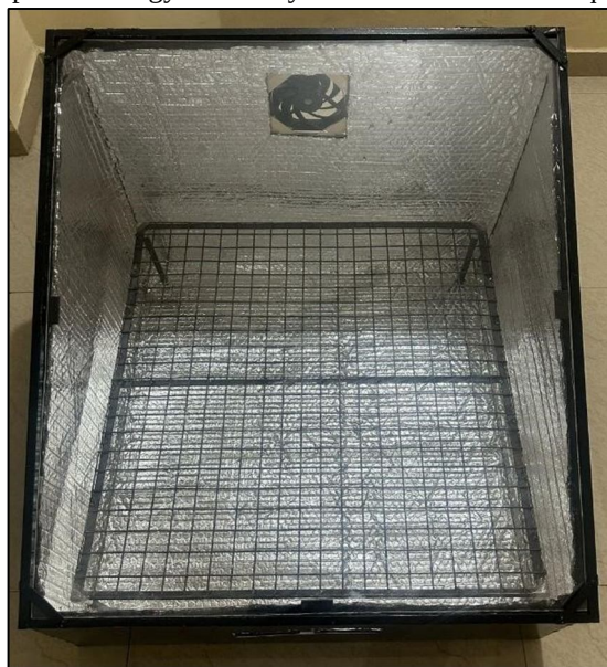
Fig. 4. Interior chamber lined with aluminum foil sheets for thermal radiation reflection.
