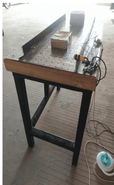
Fig : 6 : Actual IoT Based Air Conveyor System
