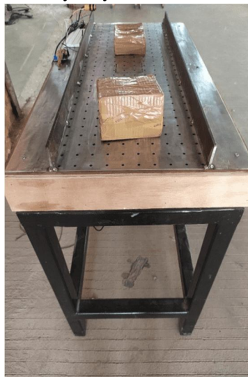
Fig : 5 : Actual Air Conveyor With Conveying Products
