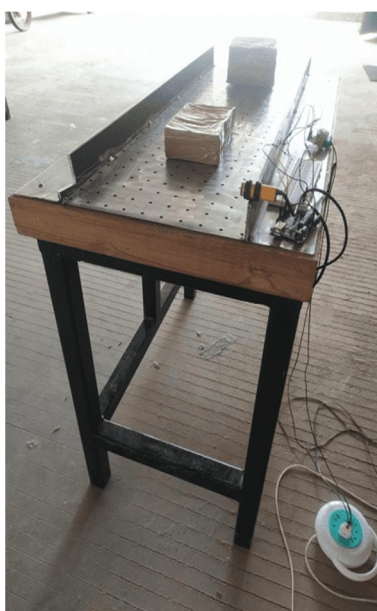
Fig : 6 : Actual IoT Based Air Conveyor System
