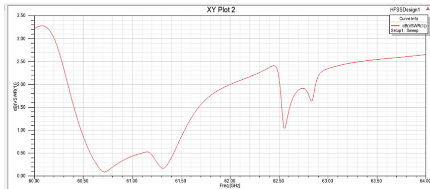
Fig. 4 Simulation result of VSWR
