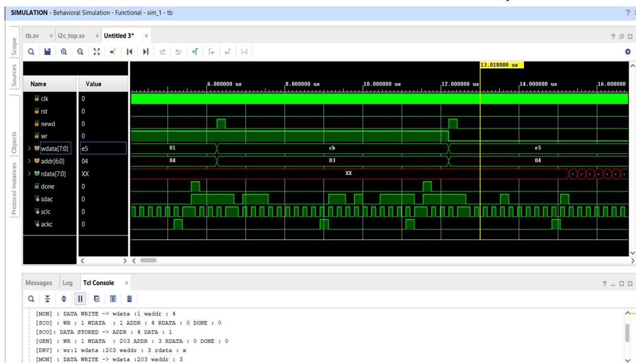
Figure 6: Behaviour of SCLclock during the read and write transaction
