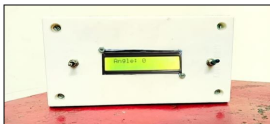
Figure 3.1 Digital Angle gauge fabricated using Arduino
