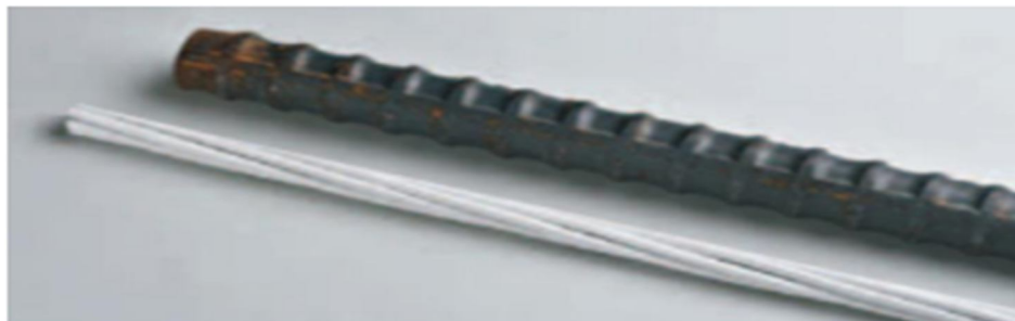
Size Comparison of Strand Rods Vs Rebar
