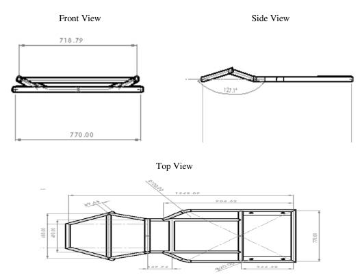
The material used to make the chassis is AISI 4130 steel. Which has good weldability, ductility, and hardness. While making this chassis we used arc welding. Chassis is the main component in kart which holds all the weight and provides suspension so it should have good hardness and should not be compromised with flexibility. The design of the chassis is done by Solid-works software as shown in fig. The weight of the chassis is 18kg
