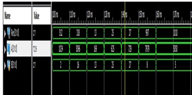
Fig : Output waveform of Divider.
