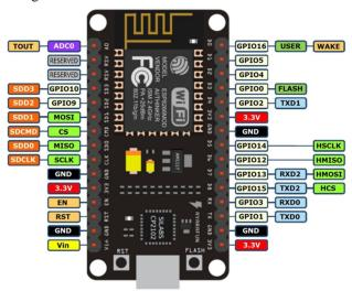
While writing GPIO code on NodeMCU, you can't address them with actual GPIO Pin Numbers. There are different I/O Index numbers assigned to each GPIO Pin which is used for GPIO Pin addressing. Refer following table to check I/O Index of NodeMCU GPIO Pins –
