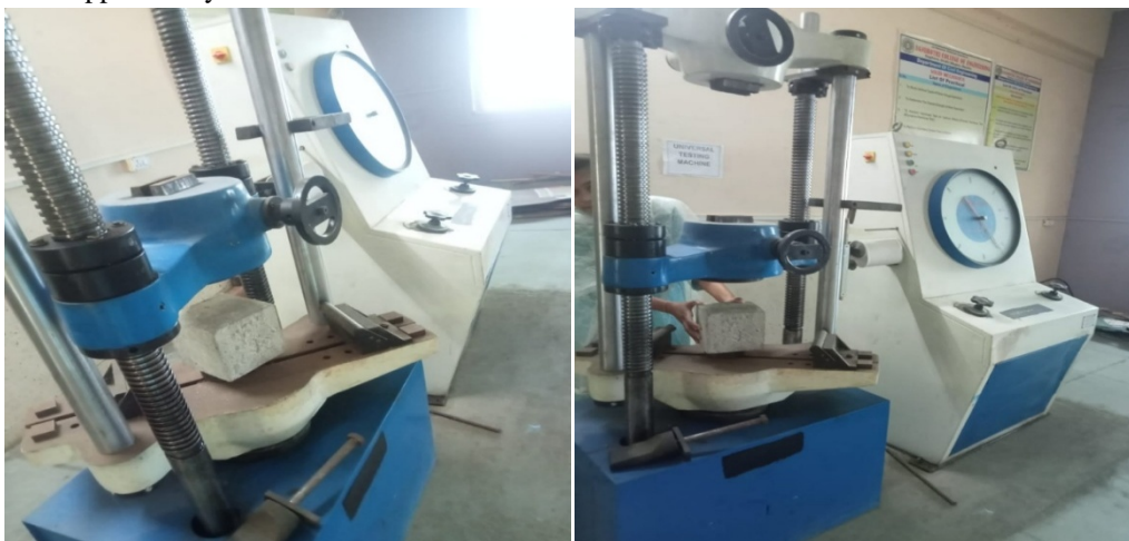
Fig.4.2: Testing of Concrete Cube by using UTM
