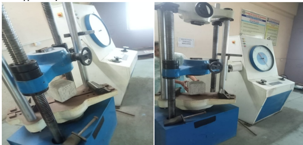
Fig.4.2: Testing of Concrete Cube by using UTM
