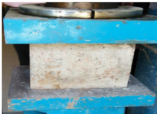
Fig.4.1: Testing of Cube Specimen in Process
