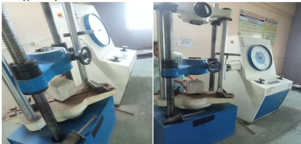
Fig.4.2: Testing of Concrete Cube by using UTM
