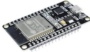
Fig : ESP32 Development Board
