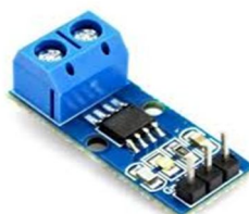
FIG: ACS712 current and voltage sensors
