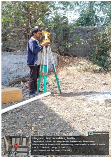
Fig. 1. First Set up Dumpy Level
