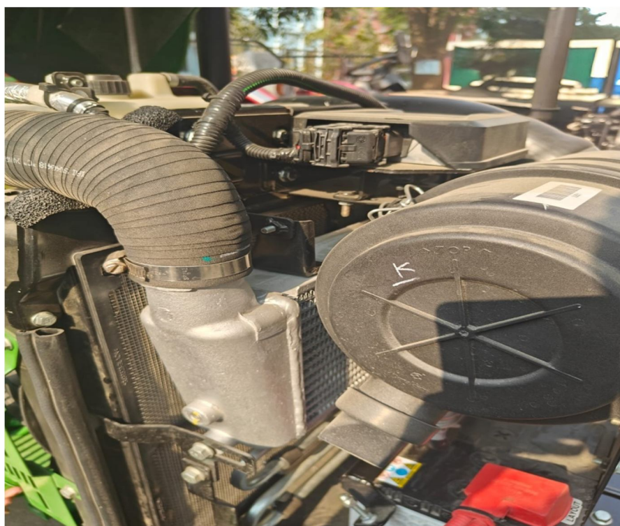
Figure 2 Side view of the radiator and coolant plumbing.
