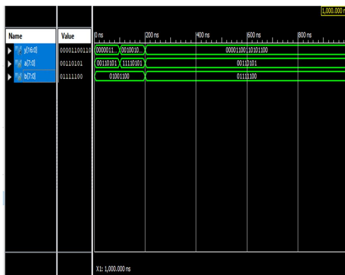
Fig 18: Simulation results of proposed Wallace tree multiplier
