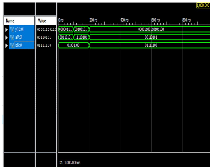
Fig 18: Simulation results of proposed Wallace tree multiplier
