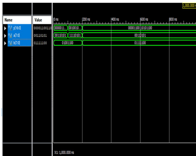
Fig 18: Simulation results of proposed Wallace tree multiplier
