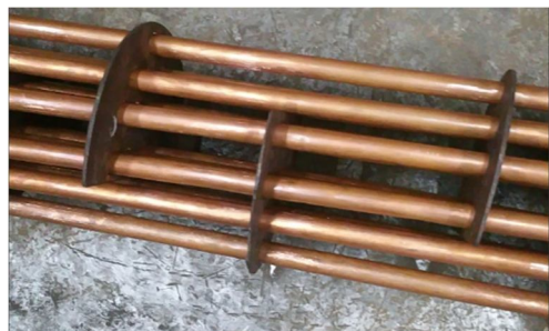
Figure 6. Copper tube with baffle plate (Manufactured)
