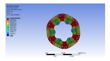
As you can see in the above model the total deformation is less as compared to the previous model.
