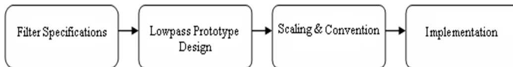
Fig3: The process of Filter design by the insertion Loss
