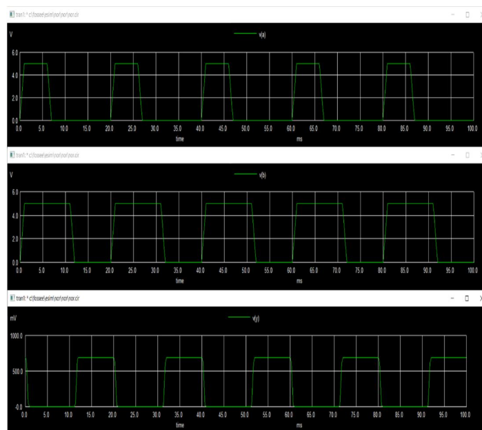
Fig.2. NOR gate NGSPICE waveform
