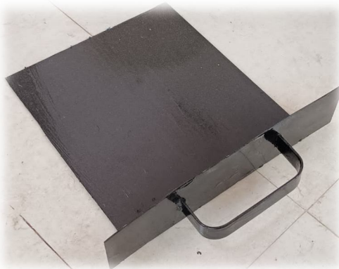
Fig. 8 Scrap inserting and removing plate
