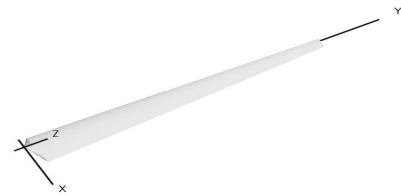
Fig. 19 Orthographic 3D view of solid blade geometry with coordinate axes linearized
