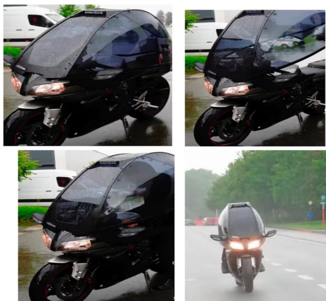
Figure 10: Reference example of a detachable, weatherproof riding shield used in international two-wheeler design. Such protective enclosures reduce wind, rain, and particulate exposure during long-distance travel, indicating the feasibility of integrating lightweight shield solutions for Indian e-scooter systems.
