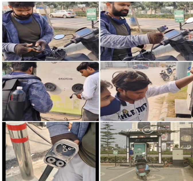
Figure 4: Attempt to charge an electric scooter at a public charging point revealing connector incompatibility and unclear plug types. The rider struggled to identify the correct interface, showing that although chargers are present, they are not designed for e-scooters, creating functional barriers for long-distance travel.
