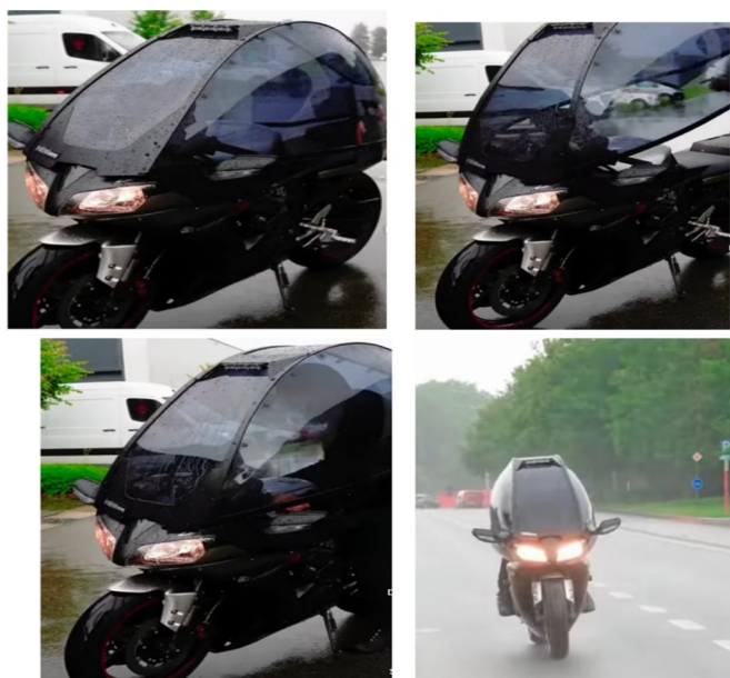
Figure 10: Reference example of a detachable, weatherproof riding shield used in international two-wheeler design. Such protective enclosures reduce wind, rain, and particulate exposure during long-distance travel, indicating the feasibility of integrating lightweight shield solutions for Indian e-scooter systems.
